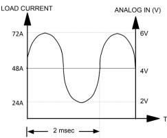
Figure 5-11: Analog Programming Example
