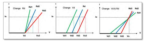
Figure 9-7: LED Based Load Curve Effects
