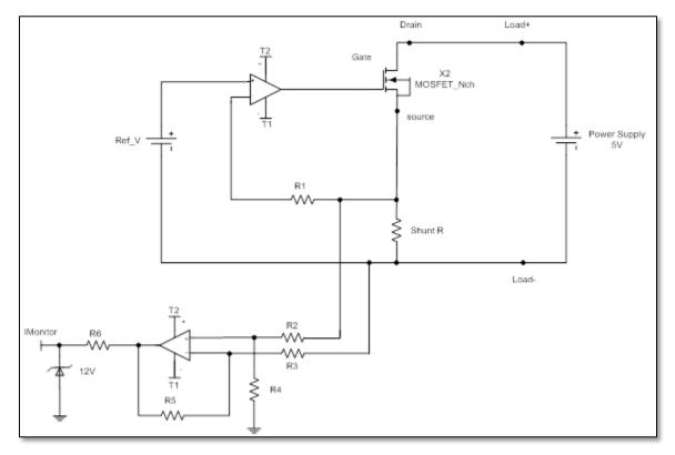
Figure 7-2: Equivalent I-Monitor Output Circuit
