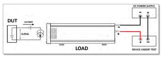
Figure 7-6: Zero Volt Load Connection
