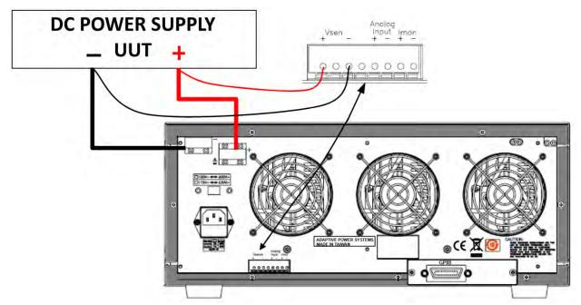
Figure 7-1: DC Load Connection with External Voltage Sense
