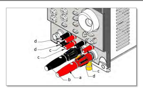
Figure 3-7: Load and sense connections using banana plugs - inserted
