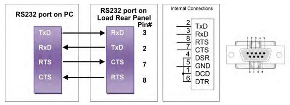
Figure 9-1: RS232 Connection to PC and DB9 Pin out
