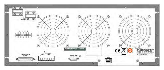
Figure 4-2: Model 5D36-24 LED Load Cabinet Master Unit Rear Panel
