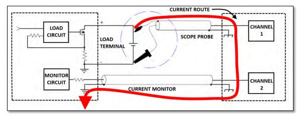
Figure 7-4: Incorrect I-Monitor Connections to UUT and Oscilloscope
