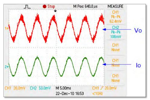
Figure 8-2: LED Voltage and Current Waveforms
