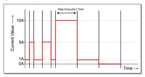
Figure 12-1: Auto-Test Sequence Example Illustration
