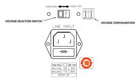
Figure 5-2: AC Input Voltage Selection
