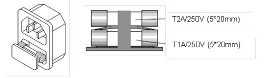
Figure 5-4: 5D18-12 Fuse Holder Location
