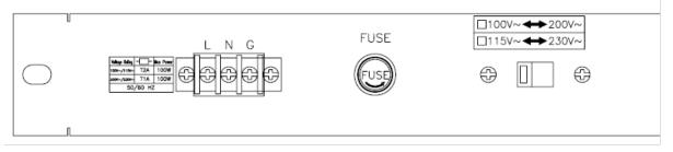
Figure 5-3: 5D36-24 Input Voltage Selector Switch Location
