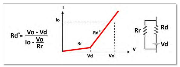
Figure 8-8: Enhanced LED V-I Curve Model
