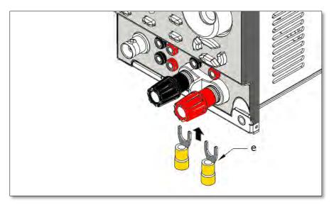
Figure 3-5: Load and sense connections using Y-hooks/spade lugs
