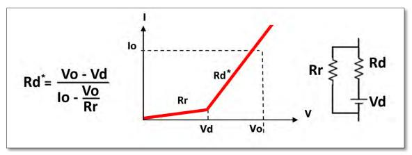
Figure 9-7: Enhanced LED V-I Curve Model
