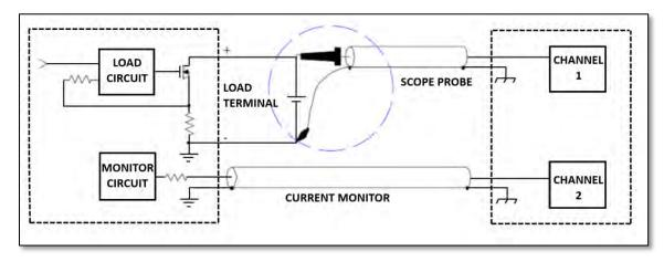
Figure 7-3: Correct I-Monitor Connections to UUT and Oscilloscope
