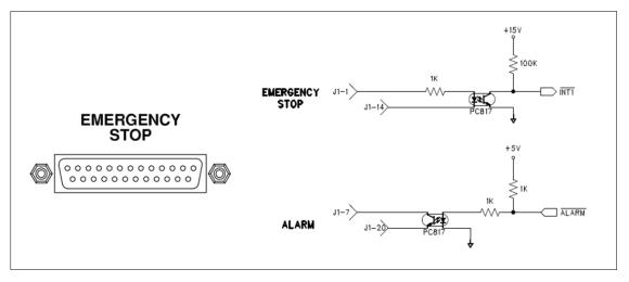
*Figure 5-13: Emergency Stop and Alarm Controller Connection*
