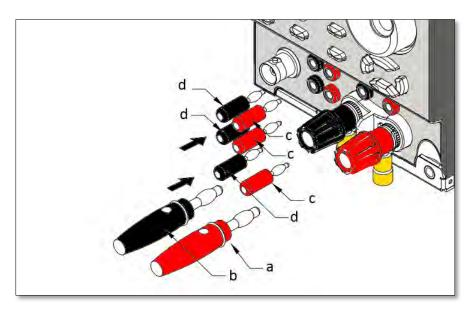
Figure 3-6: Load and sense connections using banana plugs - insertion
