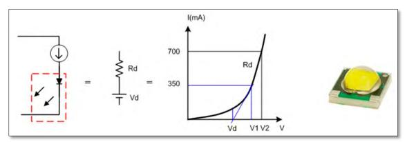
Figure 8-1: LED Equivalent Circuit Diagram
