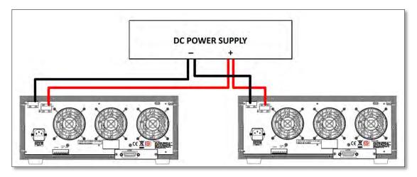
Figure 7-5: Parallel Load Connection
