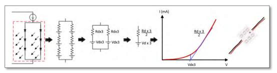
Figure 8-4: Parallel LED String Configuration
