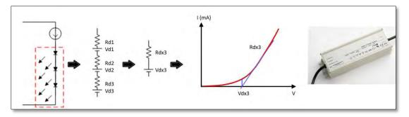
Figure 8-3: Series or Cascading LED Configuration
