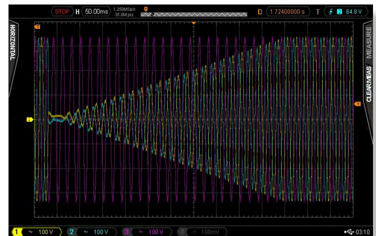
Figure 19: IEC 61000-4-34 Three Phase Voltage Variation Test
