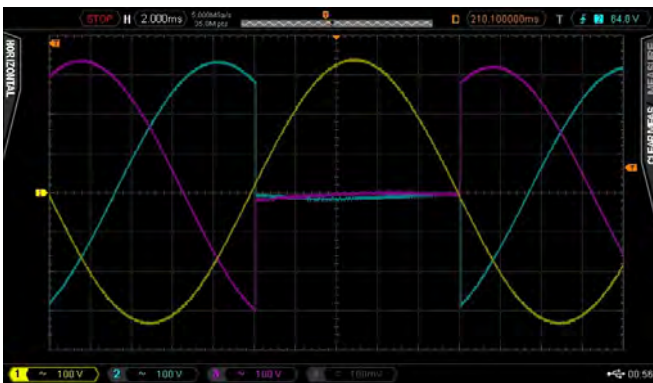
Figure 4: IEC 61000-4-11 1/2 Cycle Phase-to-Phase Voltage Dip
