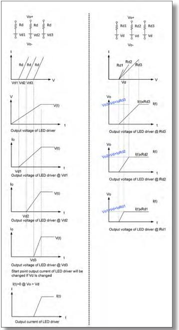
Figure 5: Equivalent LED Electrical Circuits for combination
