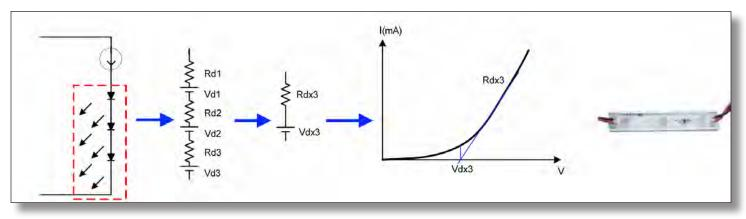
Figure 3: Equivalent LED Series String Electrical Circuit
