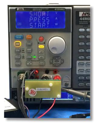
Figure 19: LED Load with shorting relay option installed
