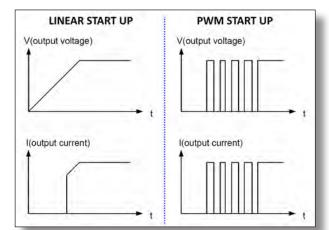
Figure 18: Linear supply versus PWM supply
