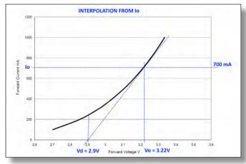
Figure 13: Tangent of forward voltage curve
