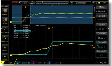
Figure 17: Start-up delayed timebase zoom
