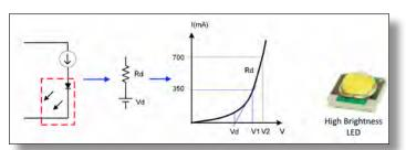
Figure 1: Equivalent LED Electrical Circuit
