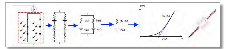
Figure 4: Equivalent LED Parallel/Series Electrical Circuit
