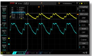
Figure 15: Checking Vo and Io levels
