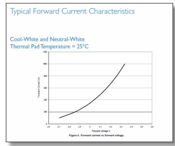
Figure 12: Philips LUXEON Rebel forward voltage chart
