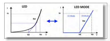
Figure 9: I-V Impedance curve for LED versus electronic DC Load in LED mode
