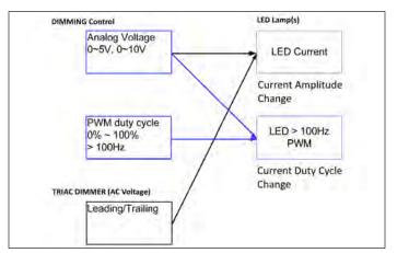
Figure 20: Varioous dimming methods
