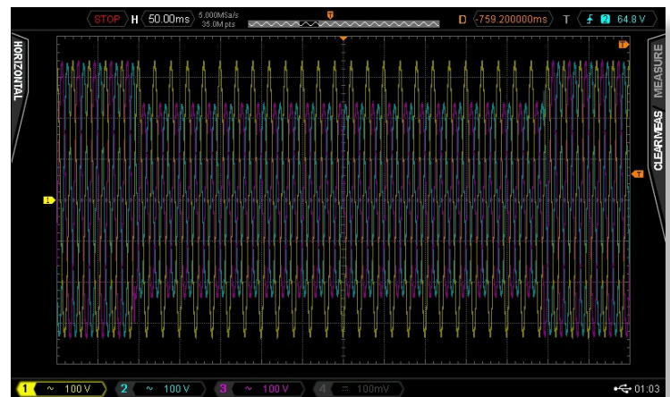
Figure 7: IEC 61000-4-11 Phase BC Voltage Dip to 70% of U_T
