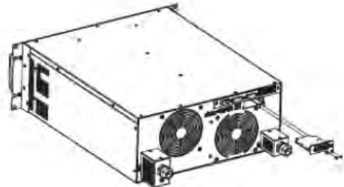
Figure 5-15: GPIB Interface Installation on 3U and 4U Models
