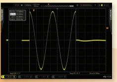
two cycle event started at 90° and terminated at 90° after two cycles.
