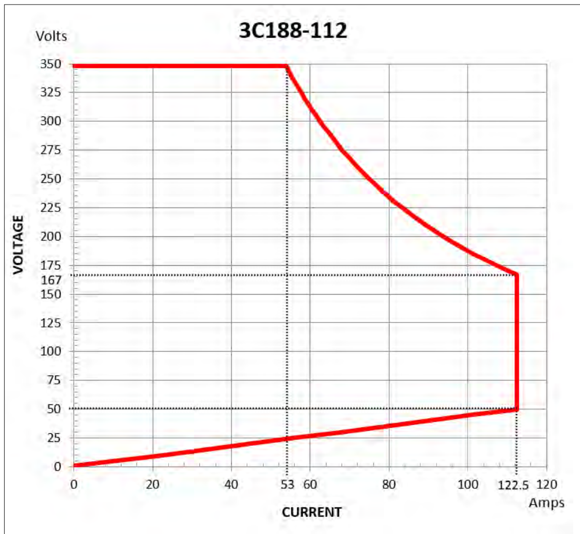
Figure 4-10: Model 3C188-112 V-I Curve
