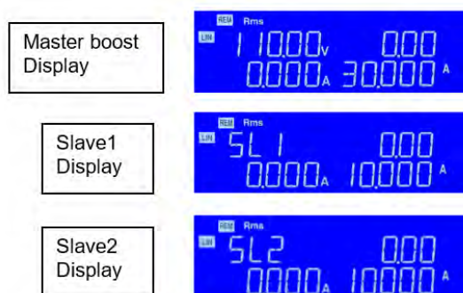
Figure 9-7: Parallel / Boost LIN Mode Setup
