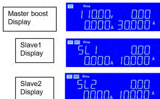
Figure 9-6: Parallel / Boost CC Mode Setup
